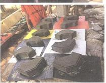
production process and eventually become a viable product. Troubleshoot issues with the community. Brick paving the product is made from sand components that are degraded from the manufacturing process, providing exceptional flexibility and fire resistance. Bring the brick from the project to the standards of the relevant Government agencies, the results are satisfactory. The price is also competitive. Importantly, all revenue from the sale is for the community to be managed to be sustainable.
